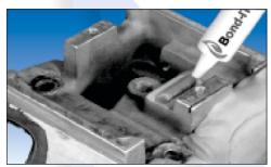
Bond-IT™ 7056AL Fills a Casting Before Re-Machining
